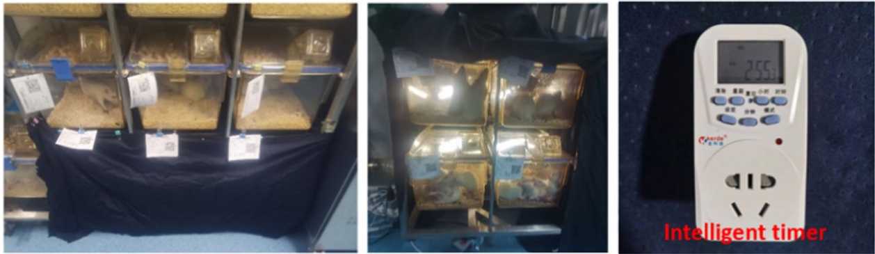
Fig. 10 Modeling of chronic circadian rhythm disruption in rats using an independent lighting system controlled by an intelligent timer
