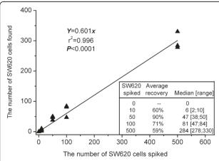
Figure 1 Calibration curve obtained by CD45 depletion in spiking experiments (n = 3) using SW620 cells at different dilutions.
