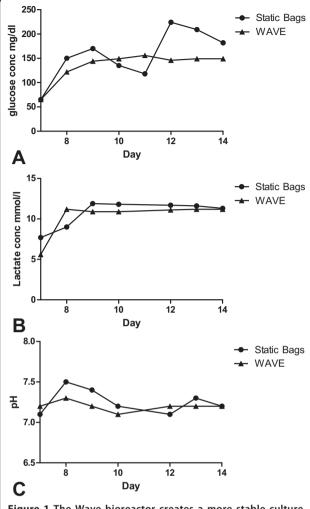
**Figure 1** The Wave bioreactor creates a more stable culture environment for rapidly expanding lymphocytes. A comparison of media depletion for a culture grown in static bags (circles) or the WAVE bioreactor (triangles). a) glucose concentration. b) lactate concentration. c) pH.
